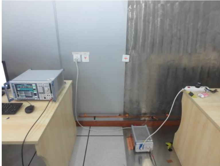
Figure 5 Conducted Emission test setup
