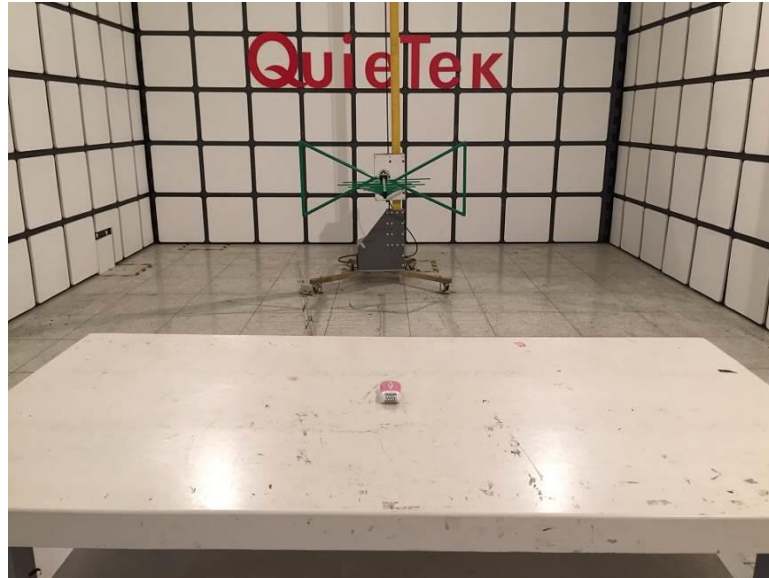
Figure 7 Radiated emission test setup
