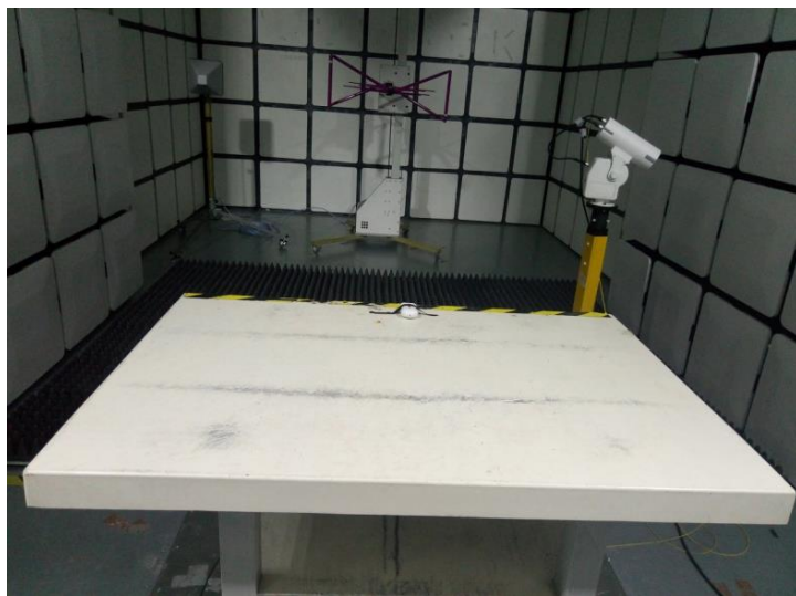
Figure 8 Radiated EM Field test setup
