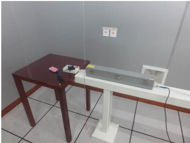
Figure 6 Disturbance power test setup
